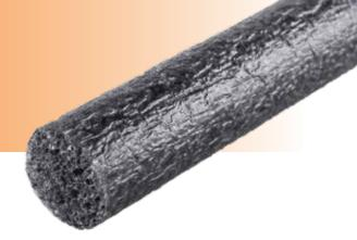
SOF® Rod is a soft bi-cellular polyethylene foam backer rod used in building envelope and concrete construction. It is comprised of both open and closed cells that will not out-gas when skin is ruptured and prevents sealant bubbling and failure.
